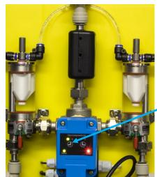
Press and hold for 3 Sec to select Actuator Valve to open Keg 1 to start.
